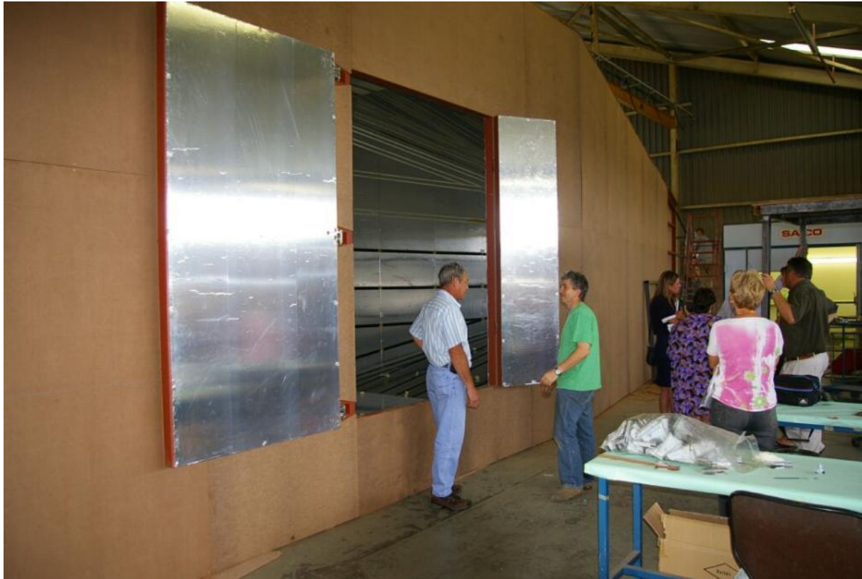
Anechoic chamber knock-down kit fully assembled
