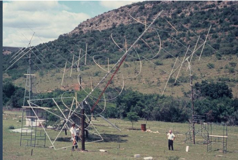
25 to 45 MHz helix at radio observatory 'antenna farm'
