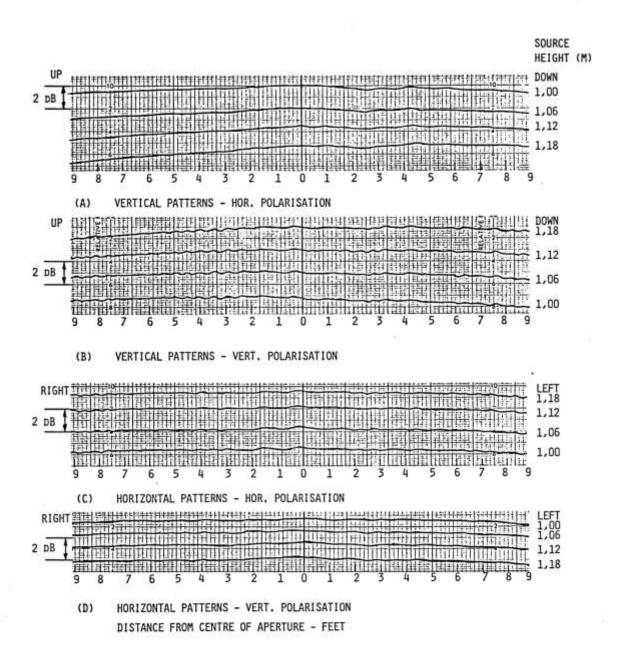
FIGURE 2: Aperture field patterns for vertical and horizontal polarisations at 2,9 GHz
