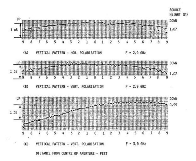
FIGURE 3: Vertical plane aperture field patterns showing predicted (• •) and measured (-----) values
