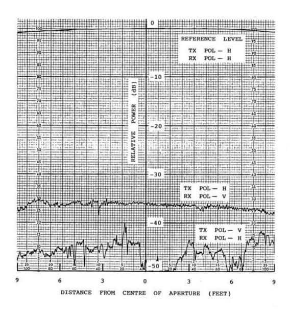
FIGURE 6: Cross polarisation level in the vertical plane over 5,5 m aperture at 9,6 GHz with  $h_{\rm t}$  = 0,35 m
