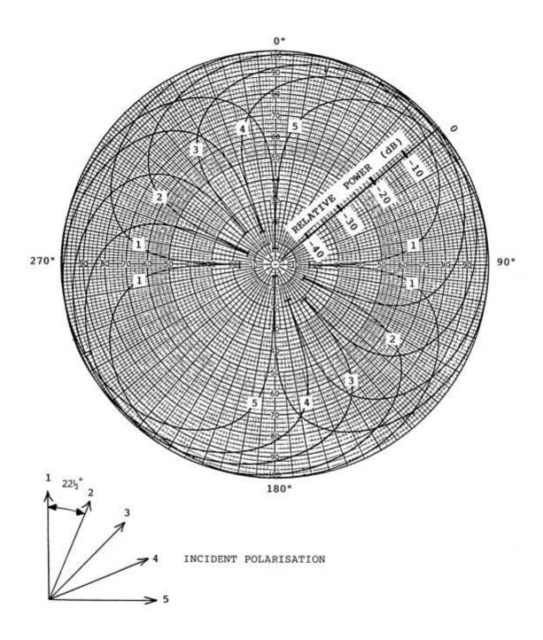
FIGURE 4: Family of polarisation patterns as a function of source polarisation angle at 2.9 GHz with  $h_{\mbox{\scriptsize t}}$  = 1,06 m
